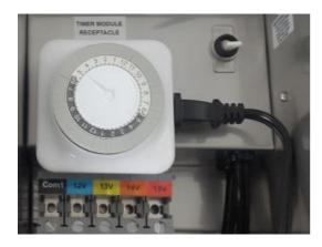
Follow the instructions for the timer to set the clock and on and off times or manually turn on/off your system.
