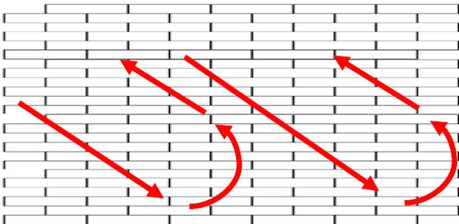
**IMPORTANT: assemble Moduline slabs and planks with an installed joint width of 1/8". Moduline spacer bars are 1/16" so it is important that the installer maintain an opening that can allow for easy jointing sand penetration including polymeric sand products. Moduline's true dimensions are based on installing with a 1/8" joint.**
