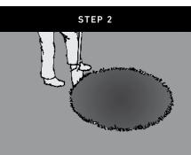
Remove all sod, roots and dirt to a depth of 2 inches inside the circle.
