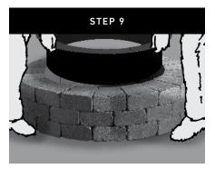
After all blocks are set, install the fire pit insert. The insert's top lip should rest on the inside edge of the fire pit blocks.
