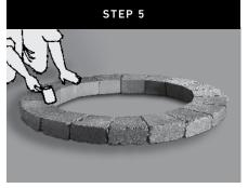
Place wall blocks on top of paver base, firmly touching each block creating a circle. Make sure each block is leveled front to back and side to side and even with adjacent blocks.
