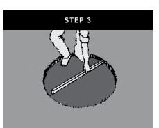
Level the soil with a tamper and remove high spots as best possible. Tip: Use a level to check.
